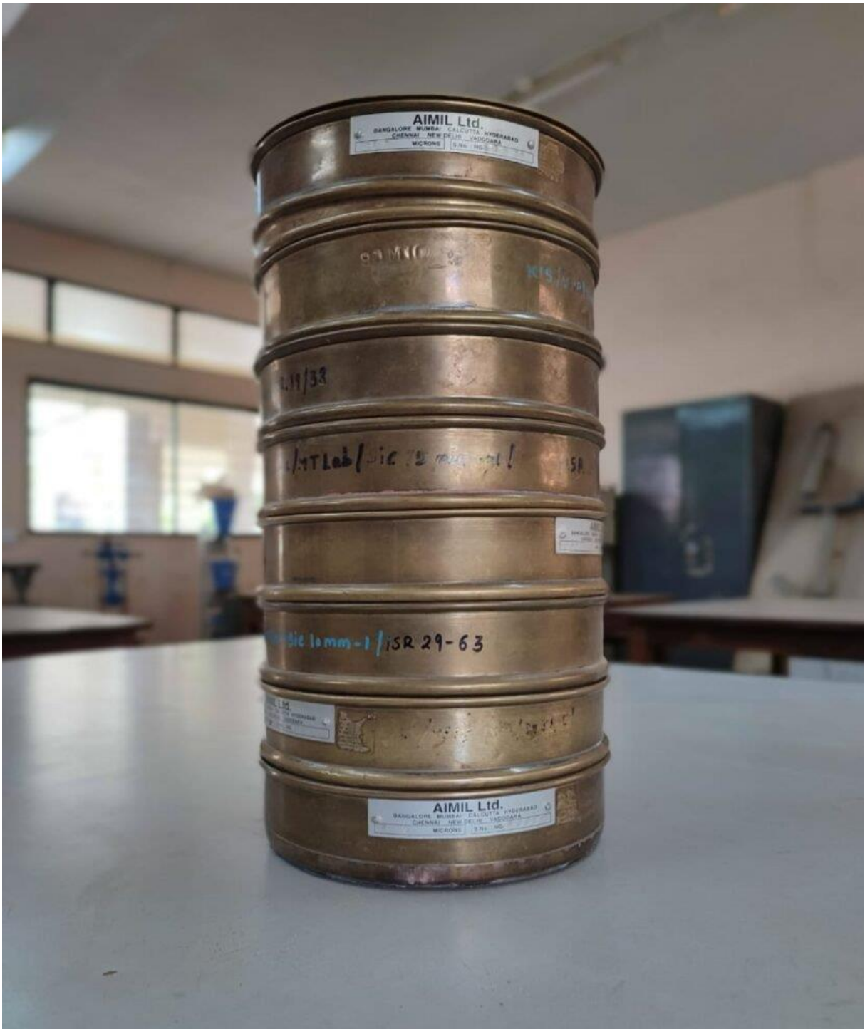
Figure 3-12: IS Sieve set from 4.75 mm to 75 micron.
