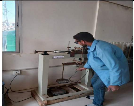
Photo Plate -8: Direct shear Test Work
