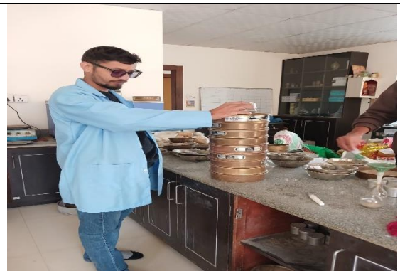
Photo Plate -6: Sieve analysis of soil work on Lab
