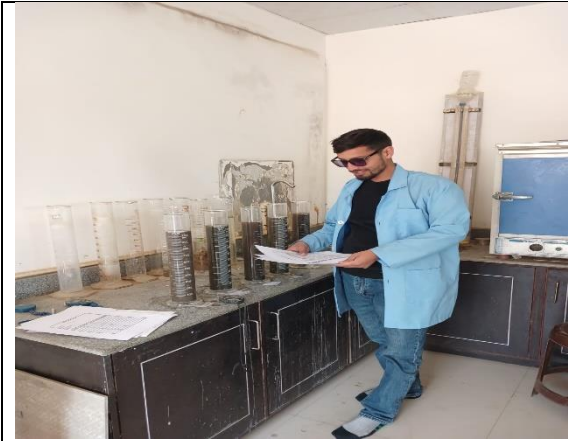
Photo Plate -7: Hydrometer Analysis Test Work
